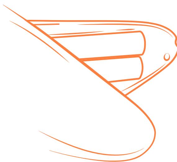
**EN** 2. Take out the old batteries and give ROMP Switch some new life with new ones. Watch out for the +/- signs.
